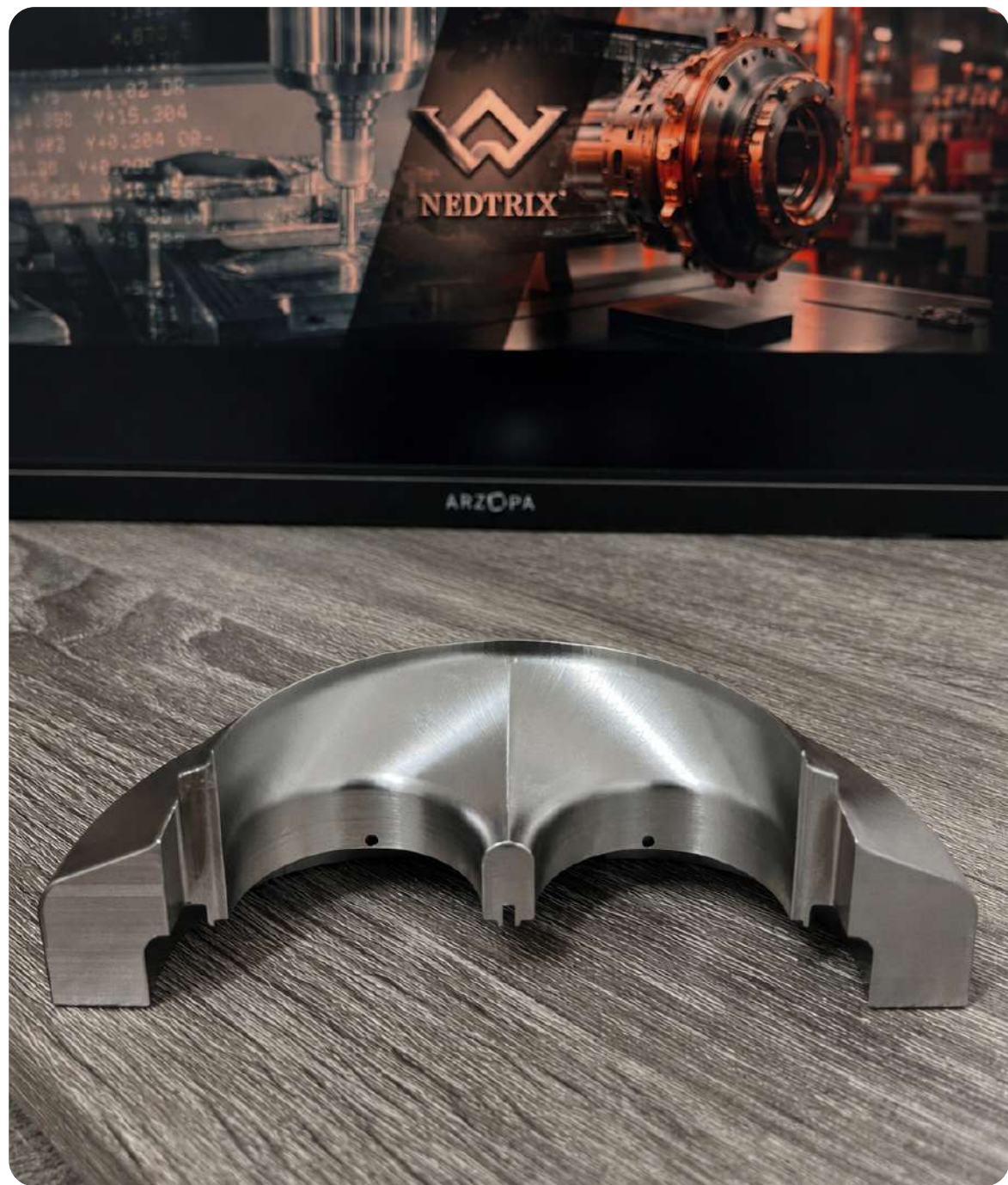
Stainless steel component manufactured by CNC milling in accordance with the customer's technical documentation.
